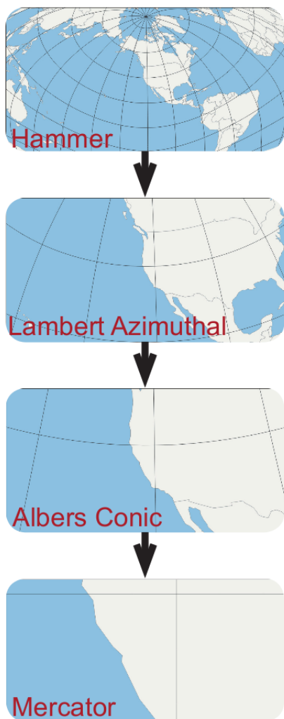
Figure 3. An example of the algorithm, zooming in on San Francisco. Note that no sharp jumps are noticeable (beyond those caused by zooming). Nonetheless, note that the graticules are straightening as we zoom in, and by the end we reach the Mercator projection, allowing us to potentially overlay tiles.
